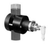
**Sight Glass Mounts** Quickly attach tubular proximity sensors to glass and plastic tubes for level detection. Often used in pairs to detect absence or presence of liquids to activate pumps and drains in process control applications.
